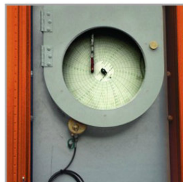
Recording instrument for tension meter
