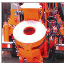
Casing rotator up to Ø 445 mm
