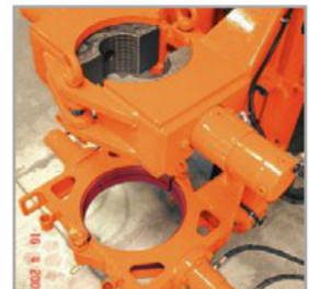
Rod clamp / Casing clamp
