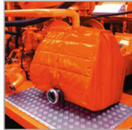
Heating jacket for piston pump
